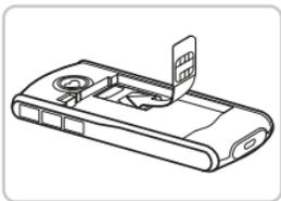
1. Remove the battery cover (opening in the top left-hand corner).
